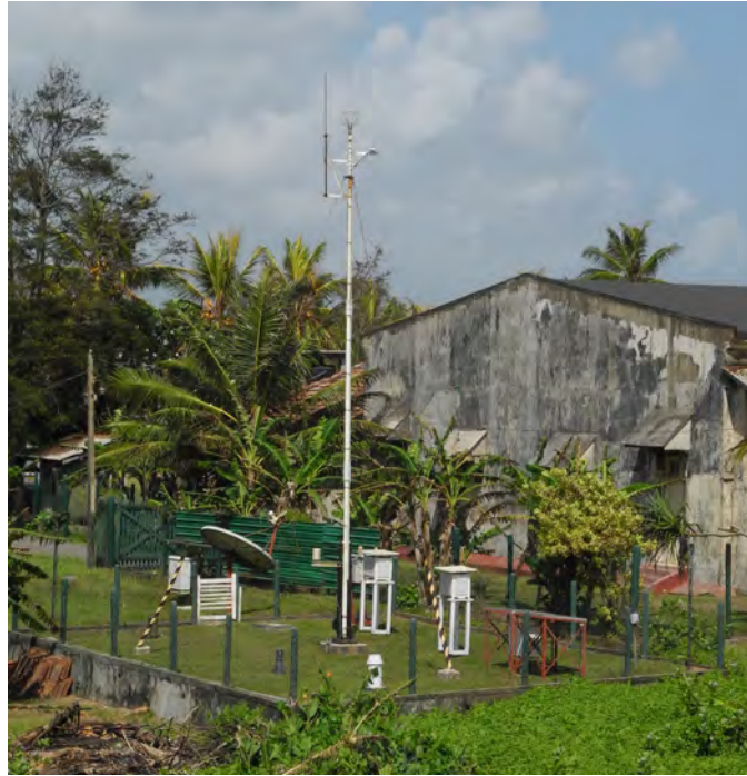
Figure 5.2: Galle Meteorological Observing Station. The tall white pole is the JICA AWS (see discussion below) while the white boxes are Stevenson Screens housing traditional instruments.
